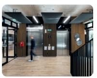
Stereo acoustic panels alternating with lighting to improve the acoustics of hallways.
